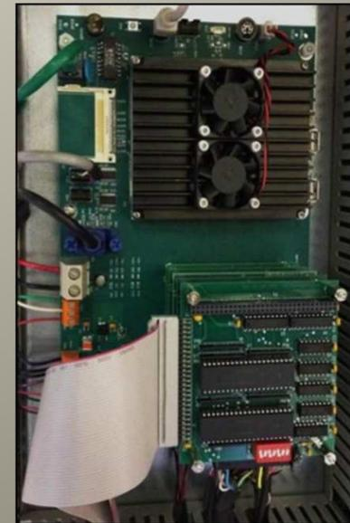
The Technician's Terminal is mounted on the front door of the MEC. The terminal is used for system configuration, set-up of measurement parameters, diagnostics, fault finding, etc.
